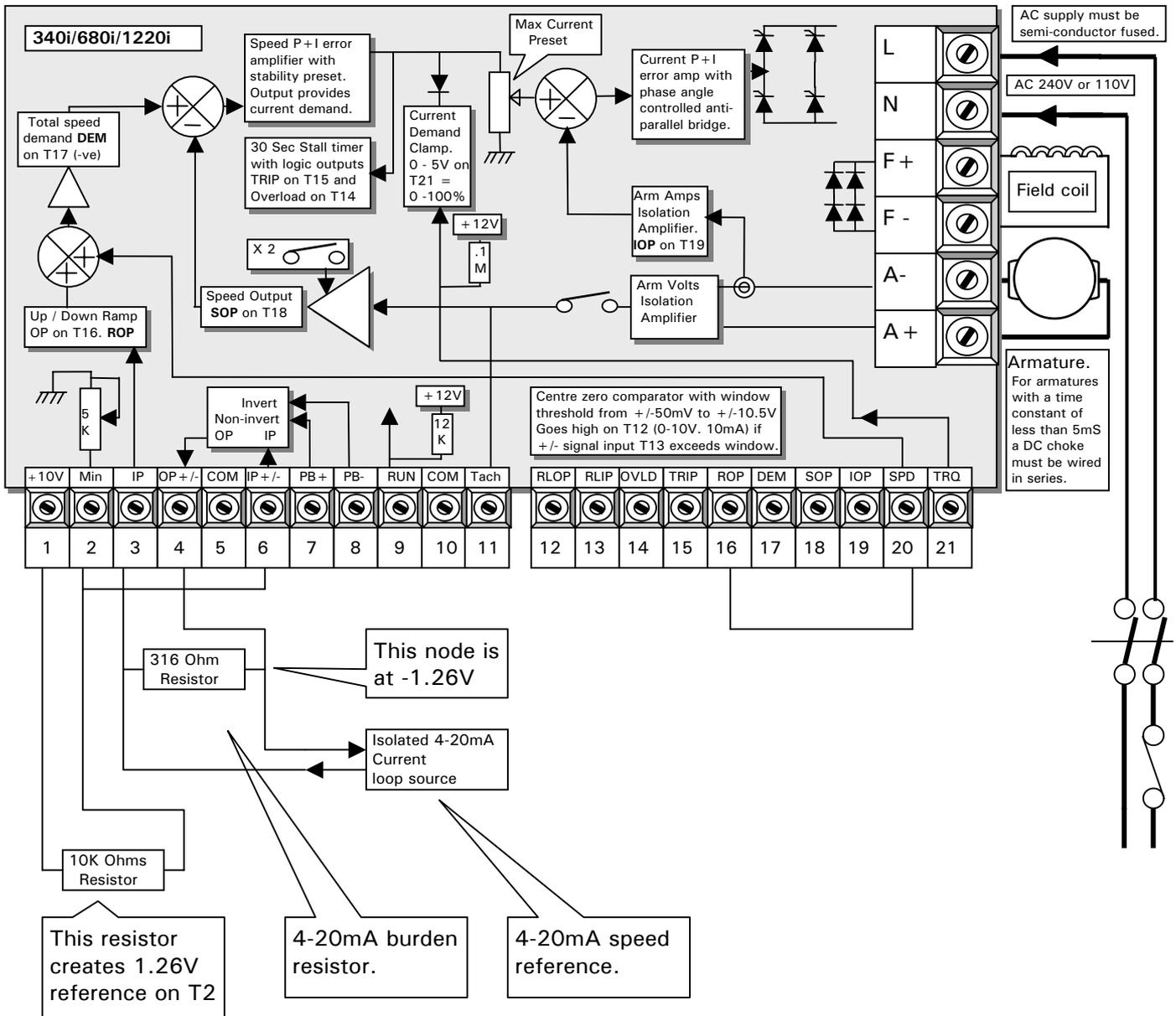
The 4-20mA floating source is imposed across a burden resistor of value 316 Ohms. (Standard E96 value). This creates a voltage of 1.26 Volts at 4mA across the resistor. This represents the system zero.
