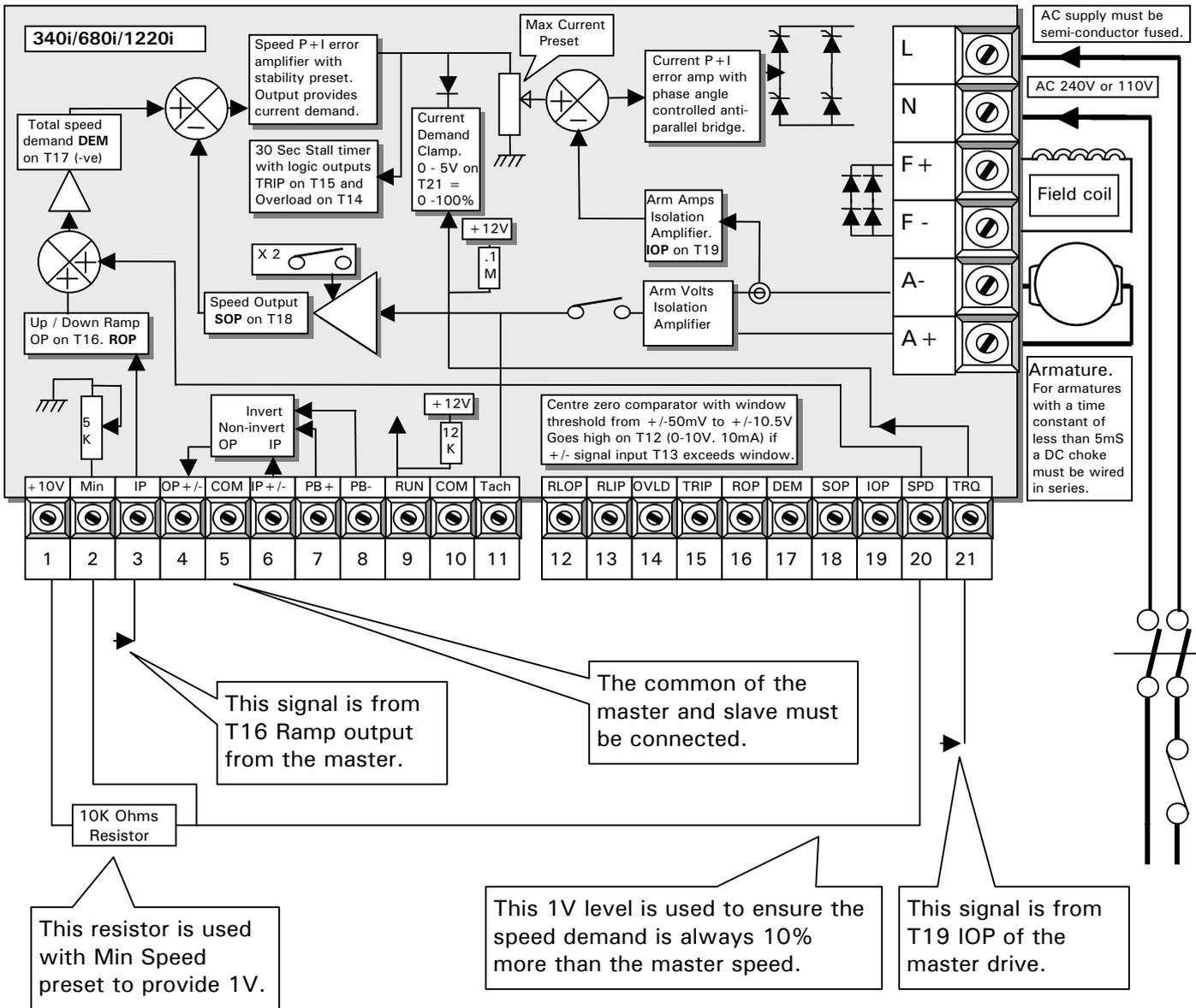
Load sharing is used when a large load is driven by more than 1 motor and each motor must bear the load in the same proportion. The motors are linked mechanically via the load and usually rotate at the same speed.
