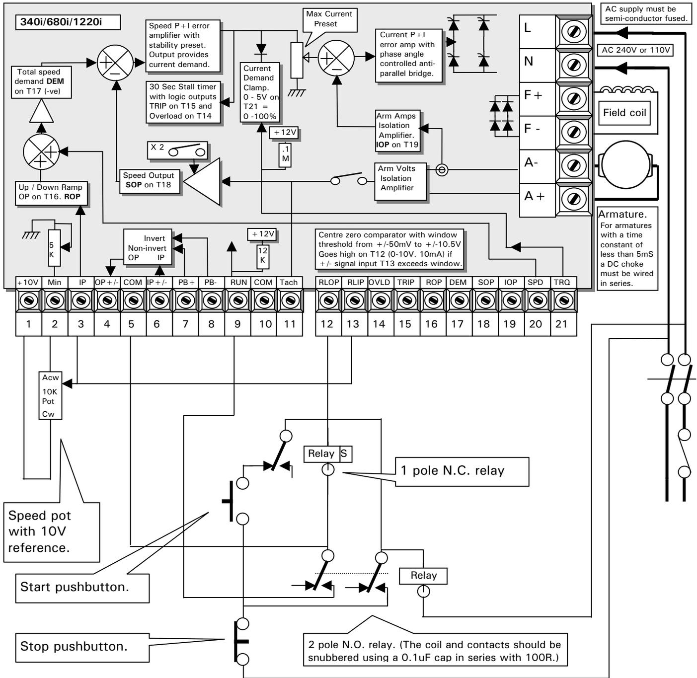
With the unit powered up and the reference above the threshold set by the relay driver level preset, the signal relay will be energised, and the contact will be closed. Hence the Start pushbutton is inoperative. When the operator brings the external reference to zero, the the signal relay will de-energise and the Start pushbutton will be operative.
