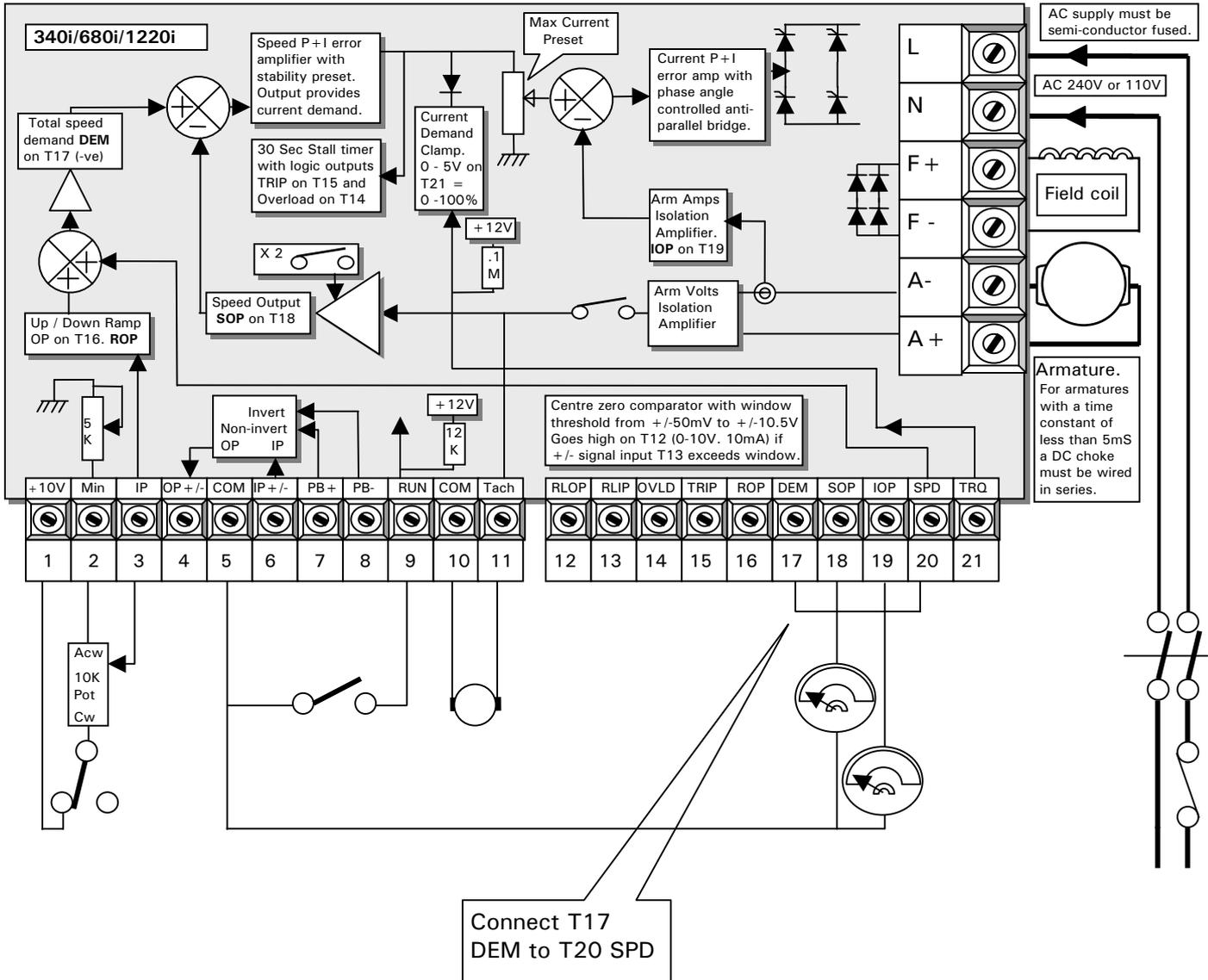
The output on T17 is the inverted total speed demand. By connecting this into T21 the feedback scaling is reduced to 50%.
