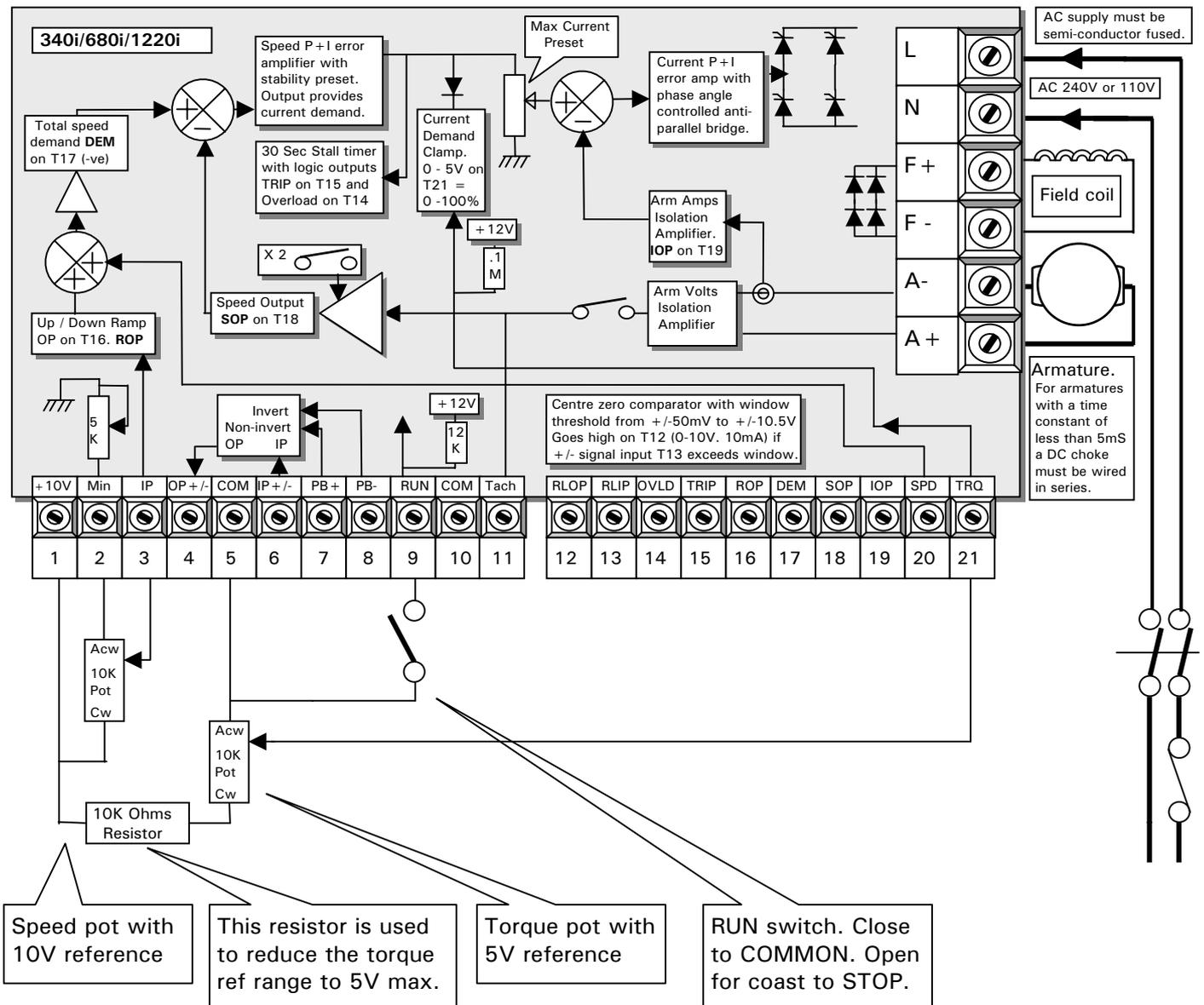
T21 is 0 to +5V input for 0 to 100% current demand. This torque signal acts as a clamp on the current demand produced by the speed loop.
