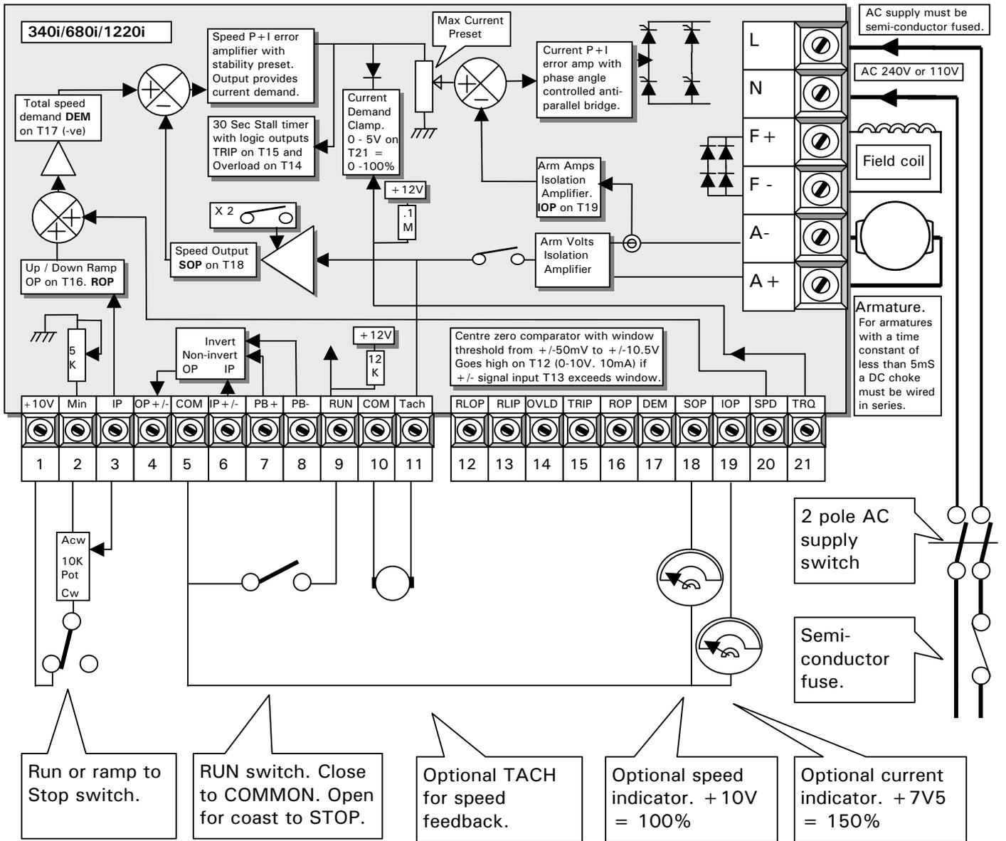
The +10V ref is connected to the speed pot by a switch giving a ramp to zero when opened.
